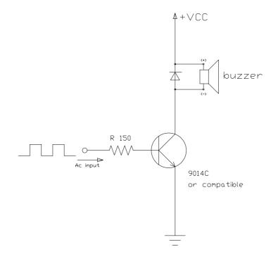
To minimize current consumption, please consider adjust its duty ratio from 50:50 to 10:90(high : low) then the consumption will decrease by about  $30 \sim 40\%$ .
