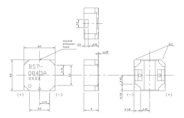
Housing Material : Nylon #46 Lead material : Gold plated Brass Weight : 0.45 grams general tolerance : 0.3 mm
