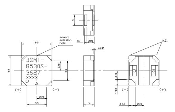
Housing Material : Nylon #46 Lead material : Tin plated Brass Weight : 0.45 grams general tolerance : 0.3 mm
