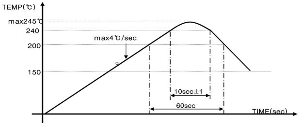
This part is able to withstand above temperature condition by 2 passes
