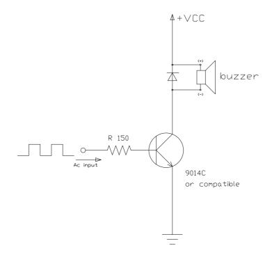
To minimize current consumption, please consider adjust its duty ratio from 50:50 to 10:90(high : low) then the consumption will decrease by about  $30 \sim 40\%$ .
