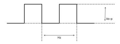
This product is designed to make its max sound when AC input signal shown in above figure with its rated voltage and frequency flows.
