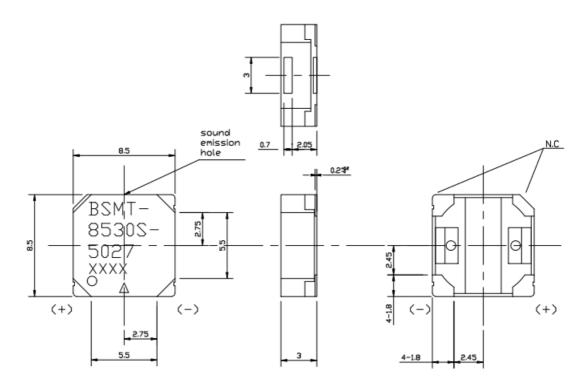
Housing Material : Nylon #46 Lead material : Tin plated Brass Weight : 0.45 grams general
