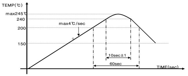
This part is able to withstand above temperature condition by 2 passes
