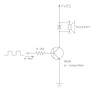
To minimize current consumption, please consider adjust its duty ratio from 50:50 to 10:90(high: low) then the consumption will decrease by about  $30\sim40\%$ .
