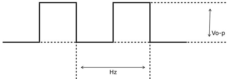
This product is designed to make its max sound when AC input signal shown in above figure with its rated voltage and frequency flows.
