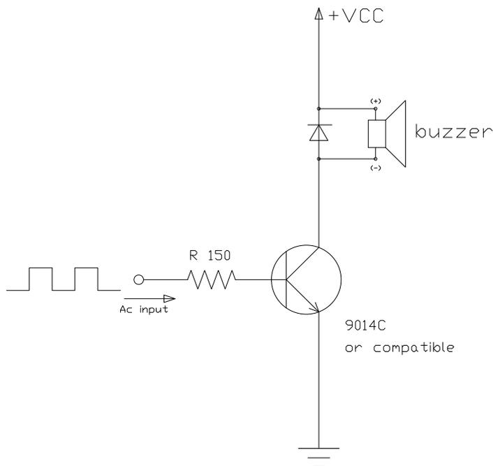
To minimize current consumption, please consider adjust its duty ratio from 50:50 to 10:90(high : low) then the consumption will decrease by about 30~40%.
