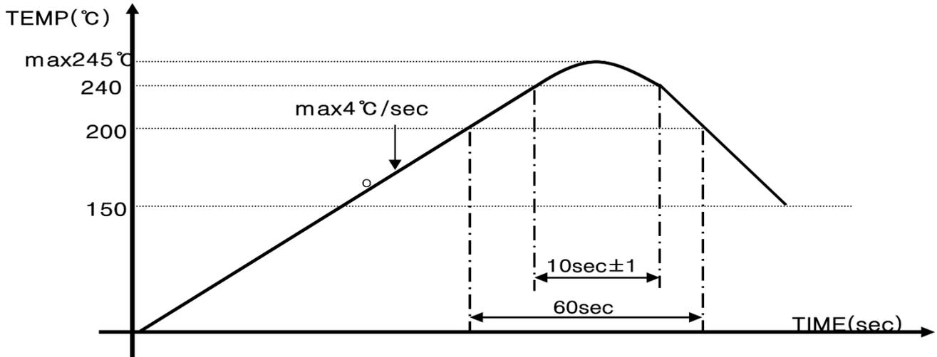
This part is able to withstand above temperature condition by 2 passes
